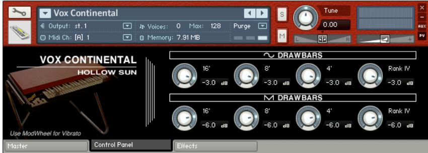
This is the meat and potatoes of all the Conti's operation, where you can set the virtual drawbars much like on the real thing. There are two sets of drawbars. One sets the levels for the sine wave drawbars and the other sets the levels for the 'sawtooth' drawbars (\*).
