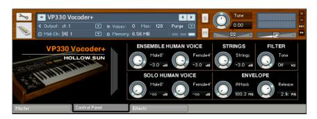
This is the meat and potatoes of the VP330's operation, where you can layer the various vocal and string sounds as well as set the overall tone and envelope shape. In many ways, this control panel offers the advantage over the original in that the the various 'layers' can be mixed in variable amounts whereas the original intruments only allowed them to be ON or OFF. The controls are:
